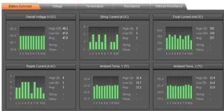
System view: View data on parallel battery strings simultaneously
